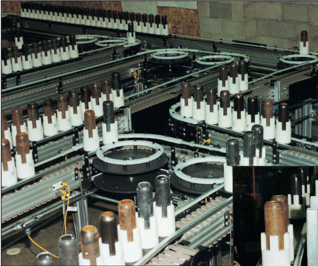
Re-orienting the product to an upright position allowed tight radius turns and conserved floor space.
