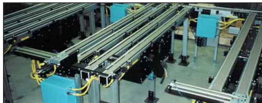
Automotive: Accumulation system with twin strand segmented belts
