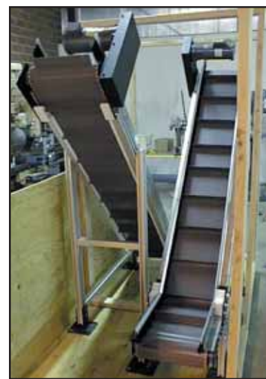
Appliance: Segmented, cleated belt incline scrap conveyors
