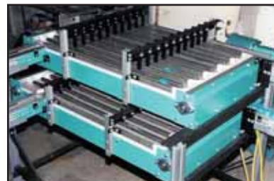
Electrical: High density, stacked serpentine part accumulators
