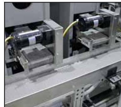
Metalworking: Low profile scrap conveyors with fine pitch segmented belts
