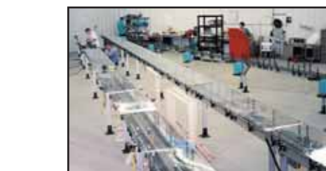
Automotive: Complete pre-assembly of inter-building transport lines
