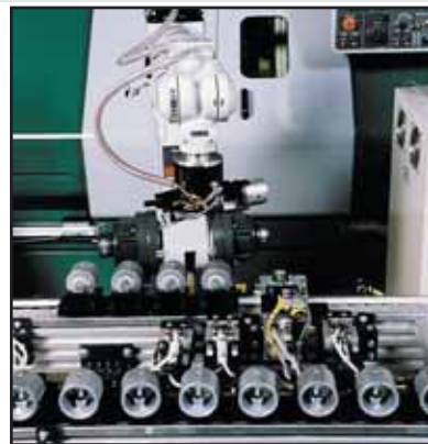
Automotive: Endless loop of 450 series conveyor with automated pallet locks
