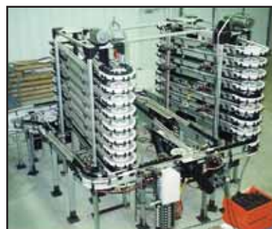
Electronics: Alpine vertical conveyors with custom part carriers
