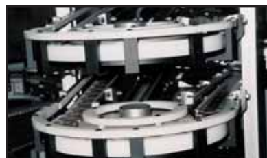
Electronics: 180-degree tight radius turn with CNC precision guiderails
