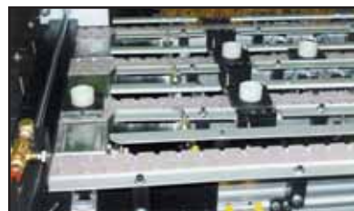
Automotive: Three low profile automatic lock stations with pallet return sweep
