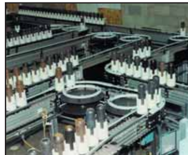
Automotive: Accumulation system of 450 series with custom part carriers
