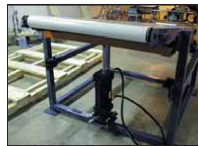
Building Materials: Belt conveyor equipped with an automatic incline actuator
